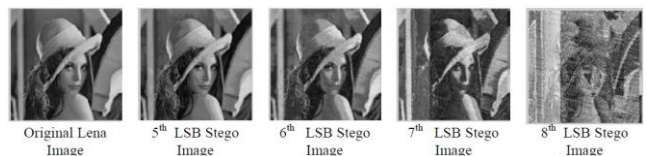
Figure 14. Cover Images and Corresponding Stego-Images using Forth LSB
